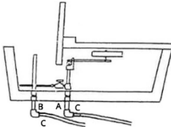
*Figure 7. Pipe Connections*
